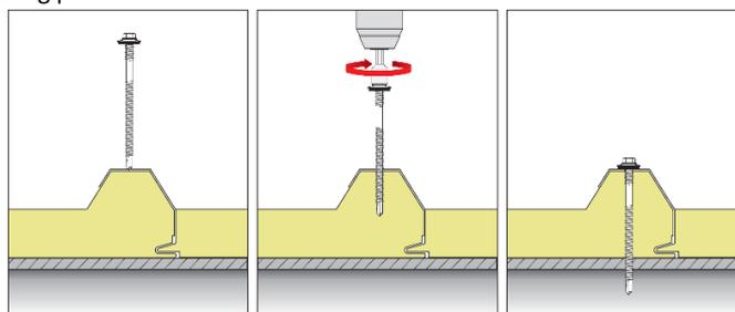
Surface mounting of roof sandwich panel (when selecting the length of the screw take into account the height of upper surface of the panel to be fixed)
